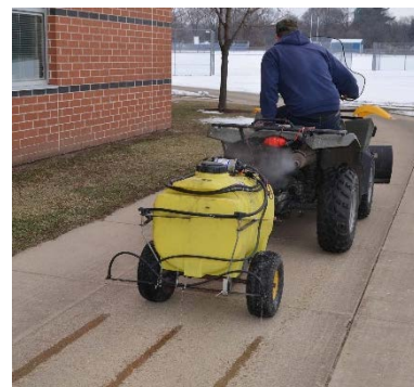
Wet/dry spread pattern equipment example; make double pass to get more lines
